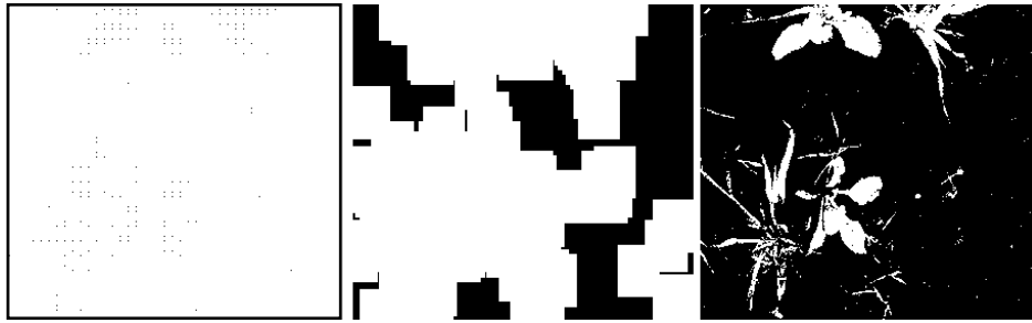
Figure 6 - From left to right: key-points from the grid, tiles around key-points and the image mask
