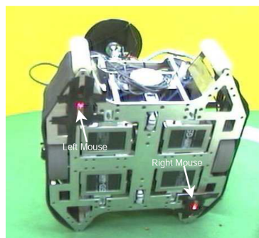
Figure 12.5: The two USB optical mice on the bottom of the base
