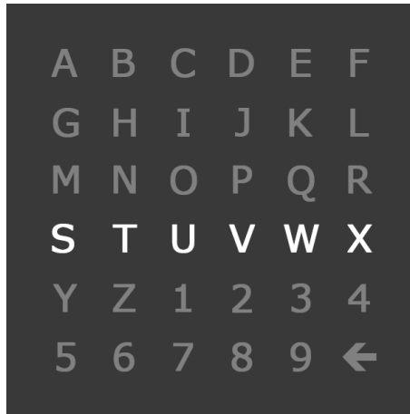
Figure 2.8: The visual stimulator for a P300-based BCI speller. Lines and rows are flashed one at a time.
