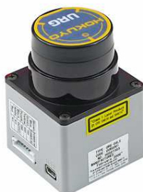
Figura 4.2: Lo scanner laser Hokuyo URG-04LX
