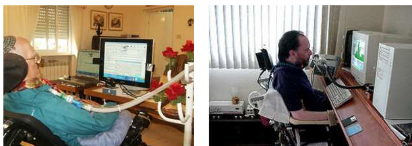
(a) ALS Patient using an eye-tracking device (b) Patient using a sip-and-puff device
