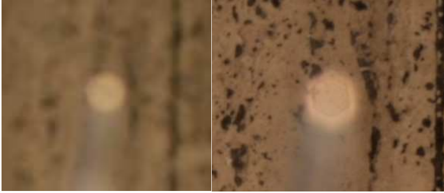
Figure 3.24: Photograph of an out of focus ballpoint pen. On the left at full aperture, the spot of light on the tip appears as a circle. On the right, aperture is reduced and the six blades of the diaphragm are visible in the PSF.
